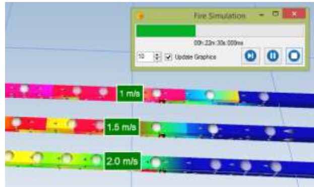
Fig. 15. VentFire™ Modelling: 1.0 m/s (top), 1.5 m/s (mid) and 2.0 m/s (bottom).
